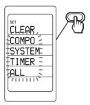
Component names are displayed on the labels. To change the labels, press the SCROLL button repeatedly. Each time the SCROLL button is pressed, the labels change as in Step 4 on page 14. 5 Select the component of which the settings you want to erase by pressing the Label Select button.
